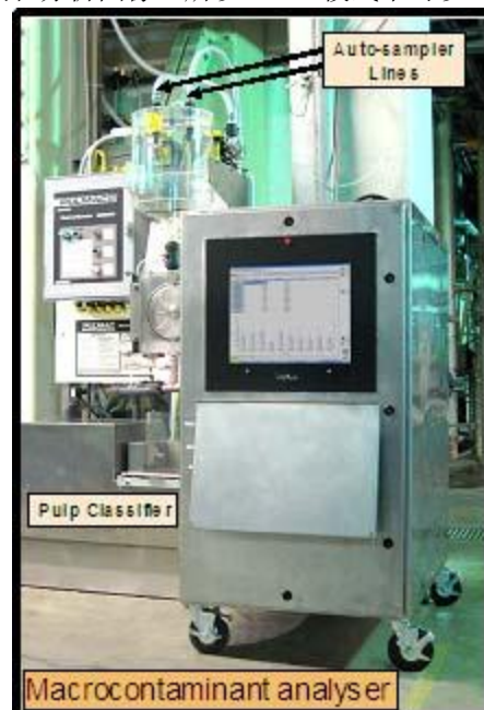
Figure 1. The analyser cabinet is in the forefront of the picture. The unit is linked to the pulp classifier and two autosampler lines.
